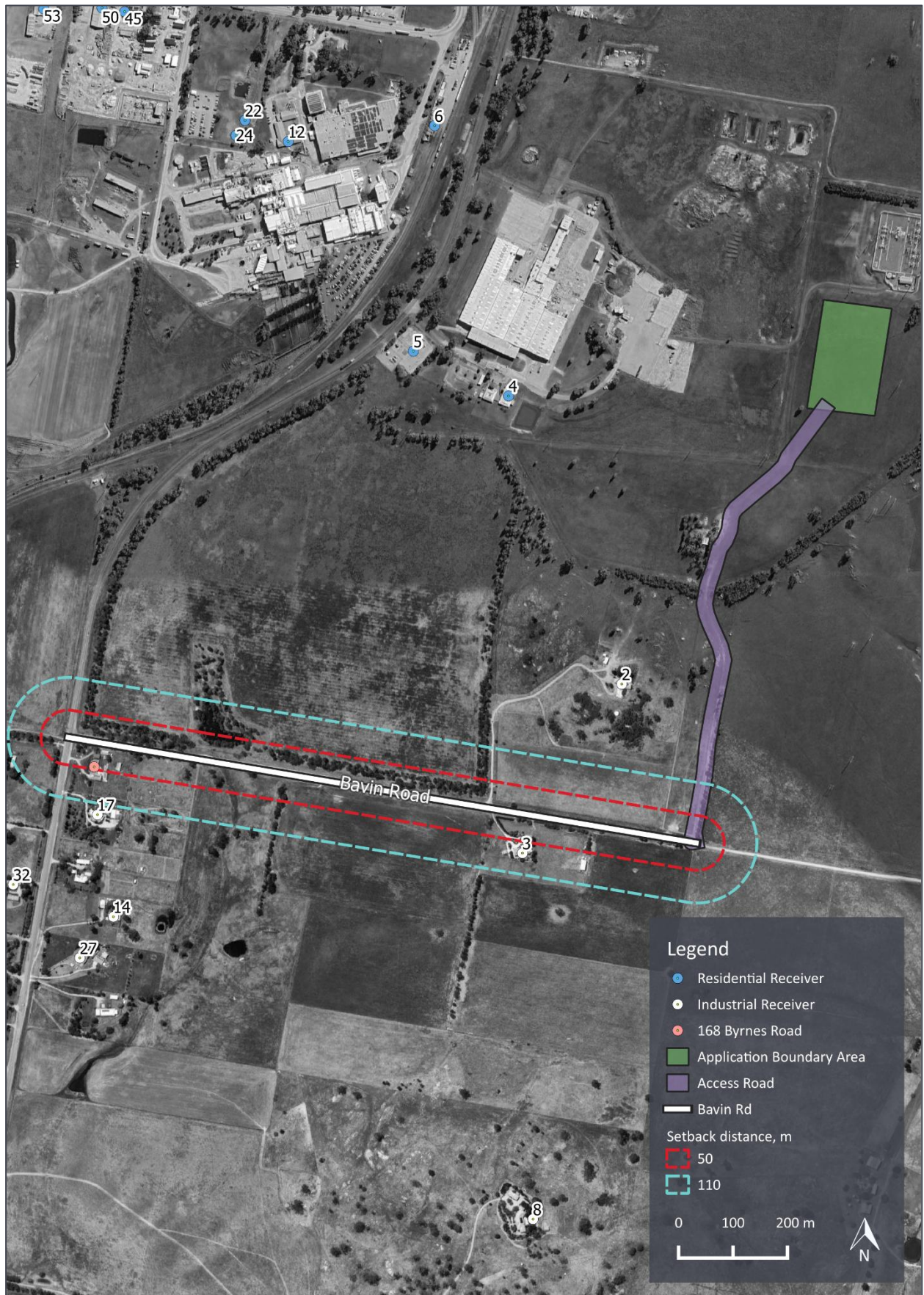
Figure 2: Receivers within minimum setback distances adjacent to assessed roads
